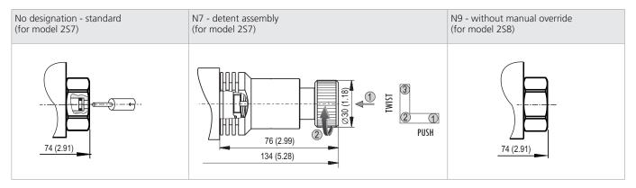
In case of solenoid malfunction or power failure, the valve poppet can be shifted by manual override under the condition that the pressure in the back line does not exceed 25 bar (363 PSI).
