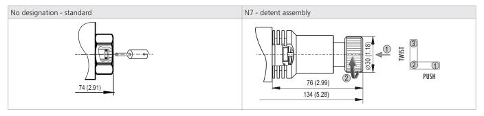
In case of solenoid malfunction or power failure, the valve poppet can be shifted by manual override under the condition that the pressure in the back line does not exceed 25 bar (363 PSI).
