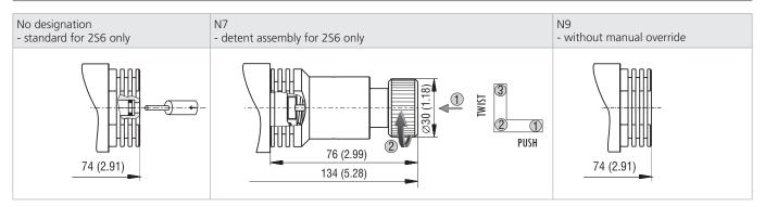
In case of solenoid malfunction or power failure, the valve poppet can be shifted by manual override under the condition that the pressure in the back line does not exceed 25 bar (363 PSI).
