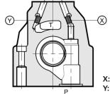
X: plug M6x8 for external pilot Y: plug M6x8 for external pilot
