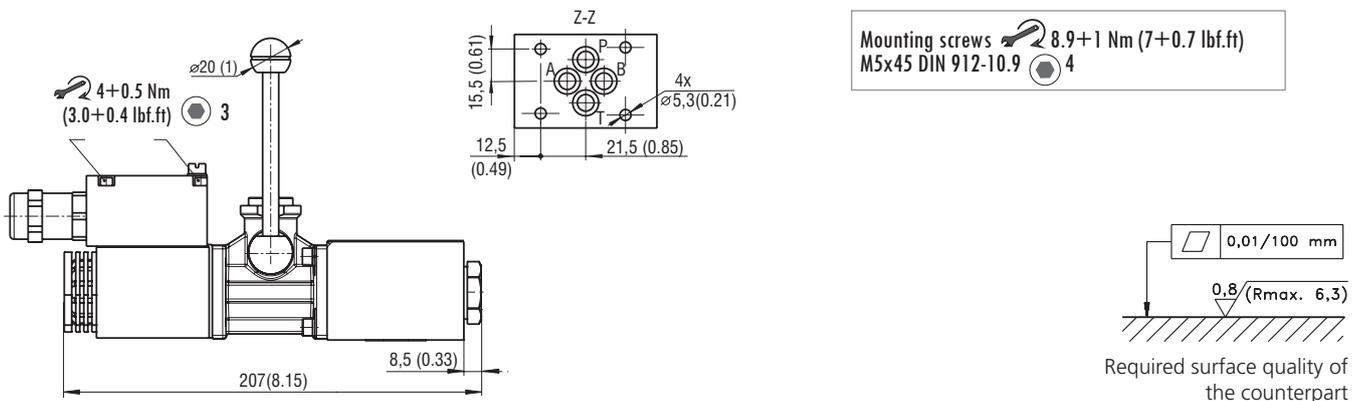
Manual lever and actuating section is shown in the standard supplied position which is the most frequently used. Both elements can be rotated to various positions 90° apart. For other positions of lever and actuating section consult our technical department for their identification.
