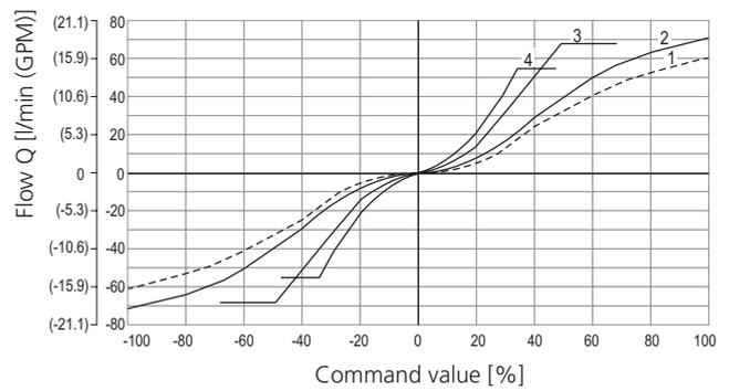
$Q_n = 80 \text{ l/min}$  (21.1 GPM) by  $\Delta p = 10 \text{ bar}$  (145 PSI)
