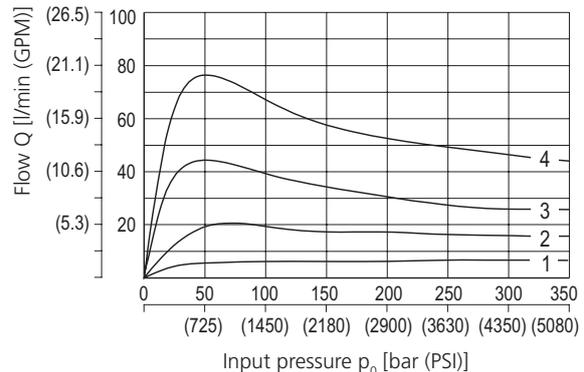
Nominal flow 80 l/min (21.1 GPM)
