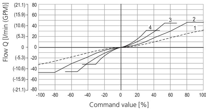
$Q_n = 60 \text{ l/min}$  (15.9 GPM) by  $\Delta p = 10 \text{ bar}$  (145 PSI)
