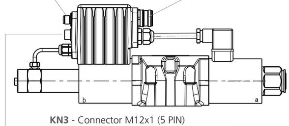
**KN3** - Connector M12x1 (5 PIN)
