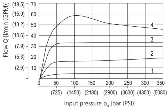
Nominal flow 60 l/min (15.9 GPM)
