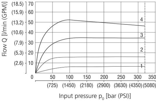
Nominal flow 60 l/min (15.85 GPM)
