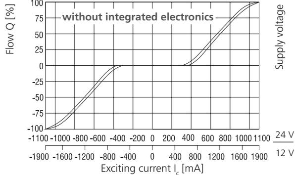
The coil current which initializes the flow through the proportional directional valve can differ due to the production tolerances about in a range of  $\pm 6\%$  of the limit current.
