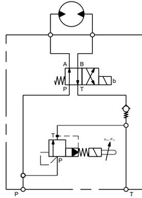
The valve is used to unload a pump to tank with a very low pressure drop. This results in less heating of the oil and therefore lower energy costs for the user.
