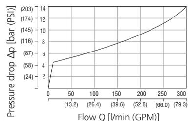
The curve refers to the pressure drop (body part only) with back pressure valve energized to which the pressure drop of the reference spool must be added.
