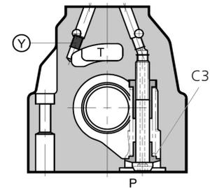
plug M6x8 for external drain
