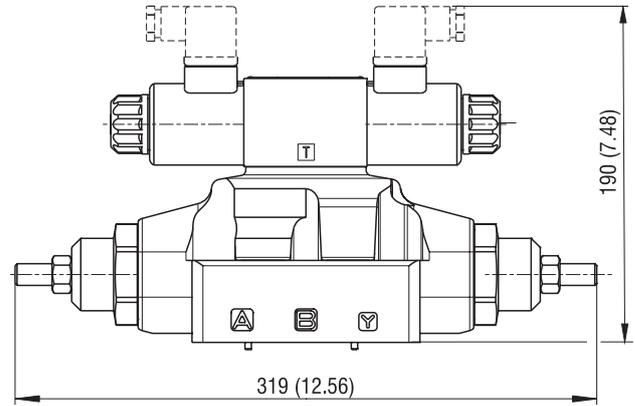
**Solenoid operated distributor with pilot valve in the configuration 3H11**
