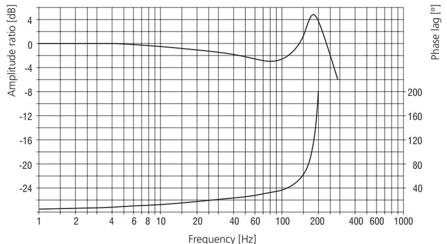
Performance Curves measured at  $v = 32 \text{ mm}^2/\text{s}$  (156 SUS) and  $t = 40 \text{ }^\circ\text{C}$  (104 °F)
