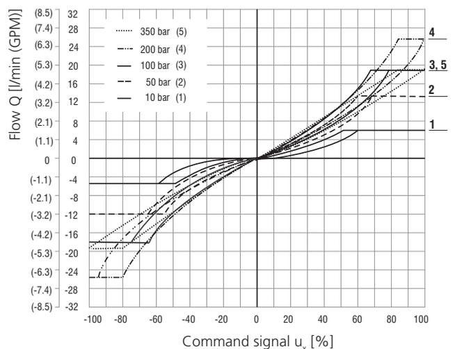
**At max current flowing through the coil 24 V (12 V), 100 % command signal**
