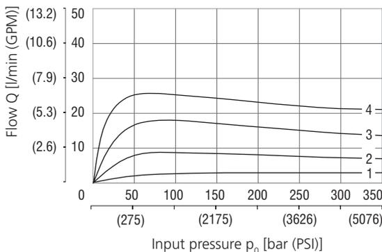
Nominal flow 30 l/min (7.9 GPM)
