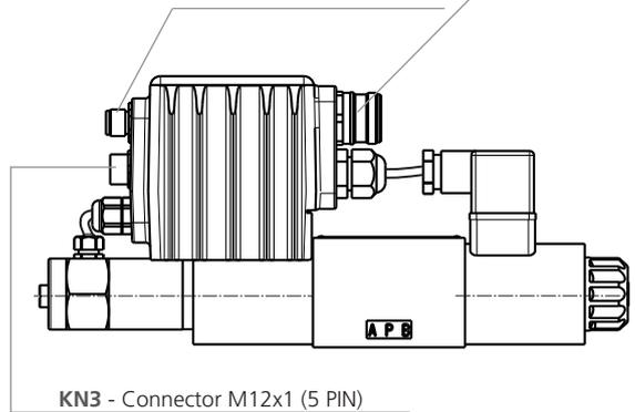
**KN3** - Connector M12x1 (5 PIN)
