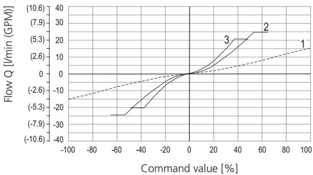
$Q_n = 30 \text{ l/min}$  (7.9 GPM) by  $\Delta p = 10 \text{ bar}$  (145 PSI)
