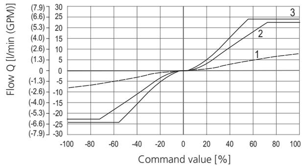
$Q_n = 15 \text{ l/min}$  (4.0 GPM) by  $\Delta p = 10 \text{ bar}$  (145 PSI)
