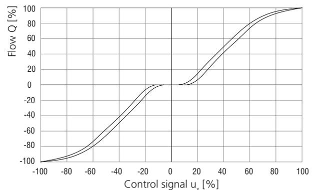
**Flow Characteristics** measured at  $v = 32 \text{ mm}^2/\text{s}$  (156 SUS)
