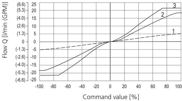
$Q_n = 8 \text{ l/min}$  (2.1 GPM) by  $\Delta p = 10 \text{ bar}$  (145 PSI)
