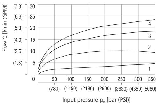
Nominal flow 8 l/min (2.1 GPM)
