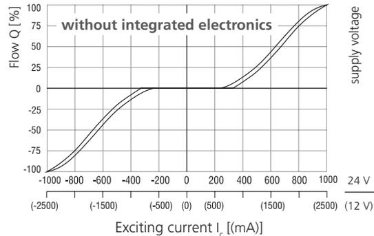
The coil current which initializes the flow through the proportional directional valve can differ due to the production tolerances about in a range of  $\pm 6\%$  of the limit current.
