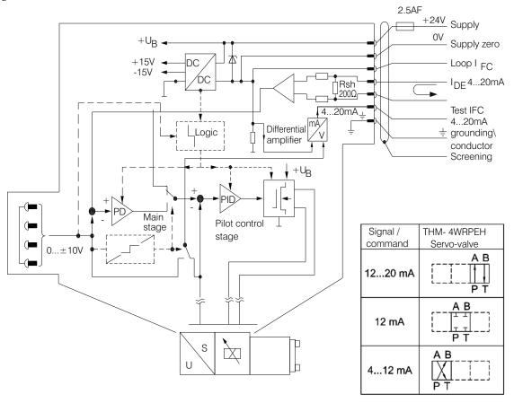
I<sub>DE</sub>≤ 2mA, Valve inactive
